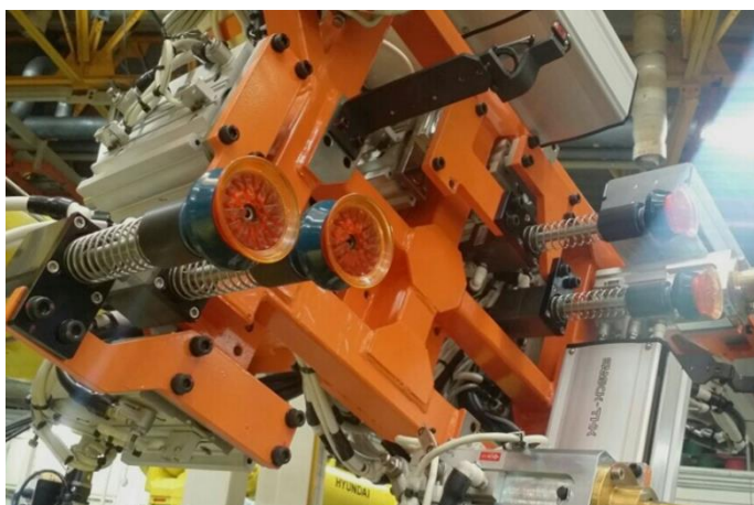
Valock system being used in automobile industry - Body line
